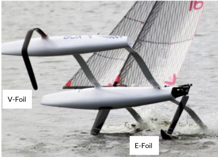
Picture of exposed hydrofoils.
